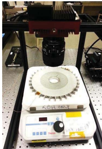
Figure 3. Setup used for both the manual translation and thermal expansion experiments. The imaging system remained the same for both experiments and only the manual translation stage and hotplate were interchanged with one another for the manual translation and thermal growth experiments, respectively.
