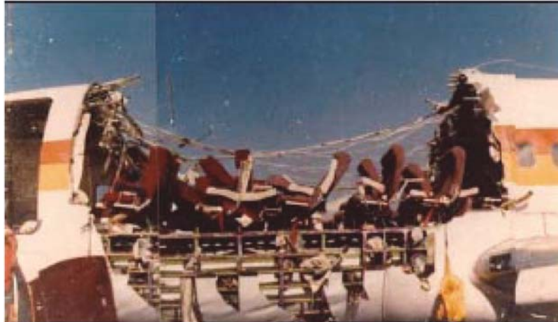
Figure 1. Wide-spread fatigue damage causes in-flight fuselage crown panel separation. Aloha Airlines, Boeing 737, April 28, 1988.
