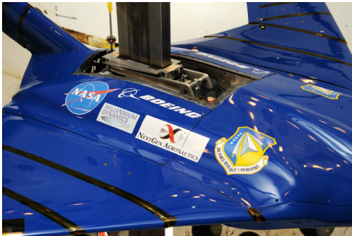
(b) Close up photograph of the joined wing model, carriage, and beam support.
