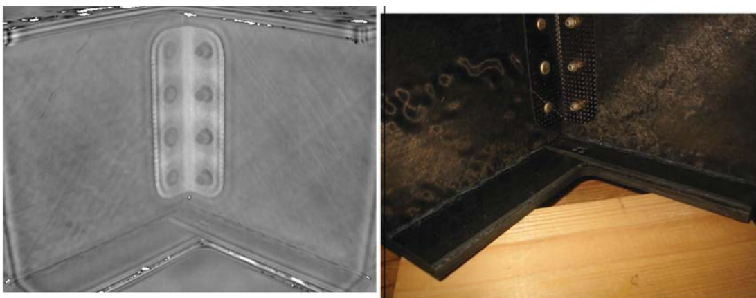
Figure A-34. Thermal inspection results for cruciform 2, rivet 4 bottom.
