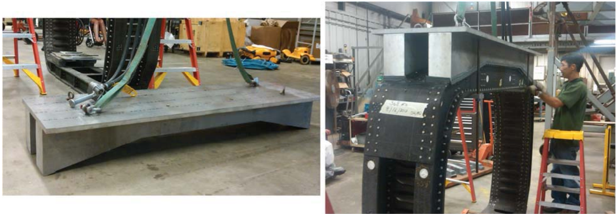
Figure 134. Photographs of aluminum blocks used to properly orient the upper mass on the fuselage section.
