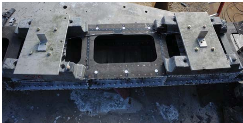
Figure 73. Post-test photograph showing the interior of the floor.
