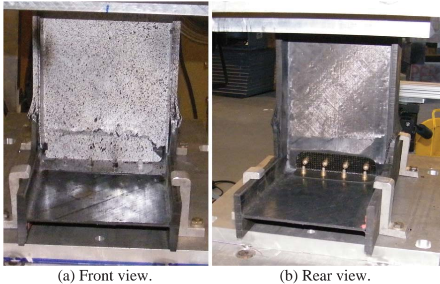
Figure 24. Post-test photographs of the 2-ft T-section test specimen.
