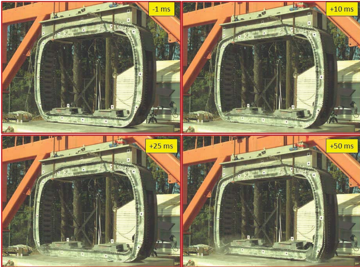
Figure 64. Image sequence of the fuselage section drop test from the southeast camera.
