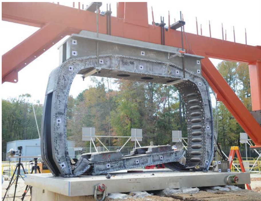
Figure 70. Post-test photograph of the framed fuselage section test article.
