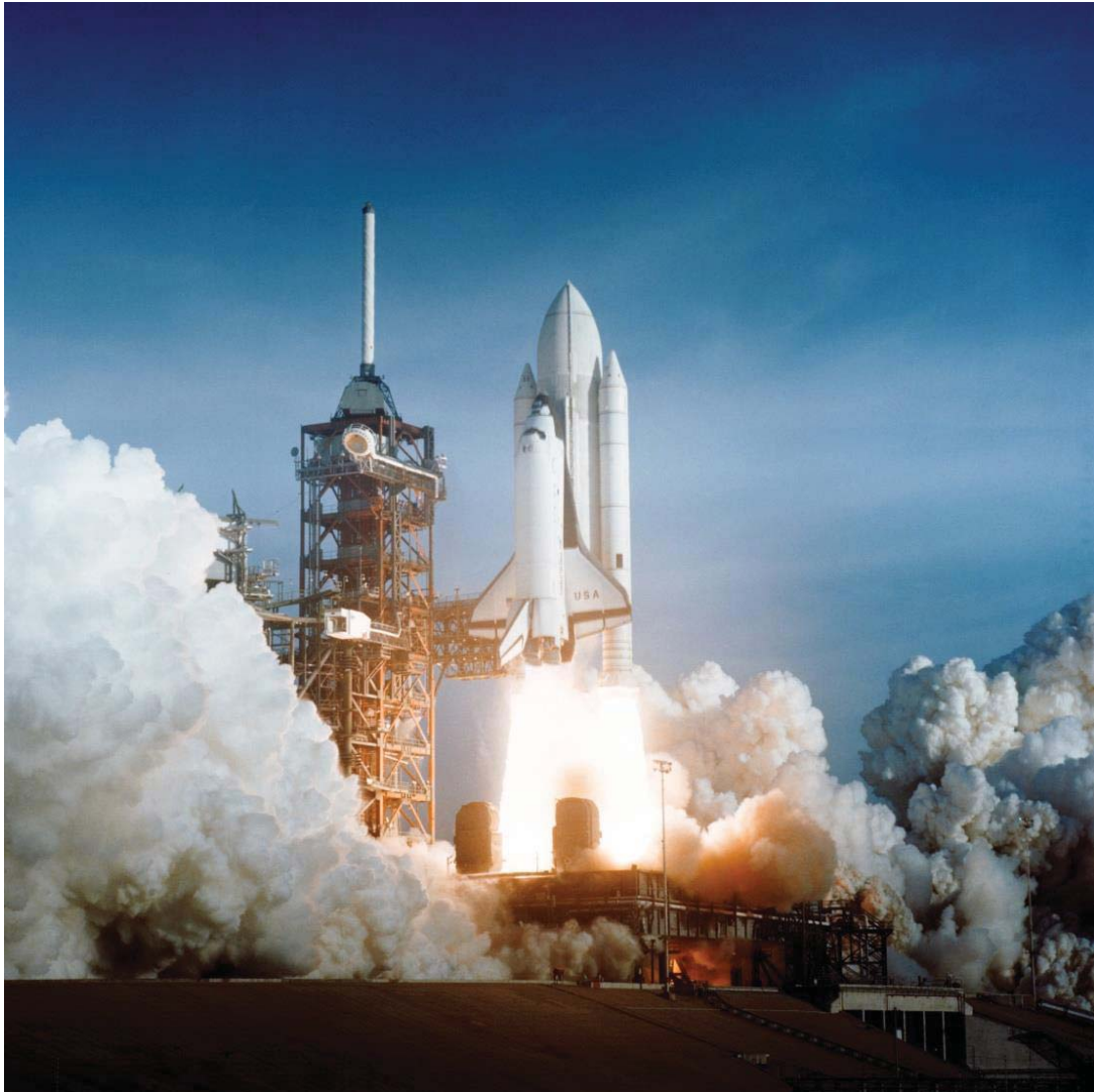
Figure 1. Launch of the Space Shuttle (STS-1) on April 12, 1981. A deflector in the flame trench beneath the mobile launch platform directed the shuttle main engine exhaust to the south (left) and the solid rocket motor exhaust to the north (right) of the pad away from the vehicle.
