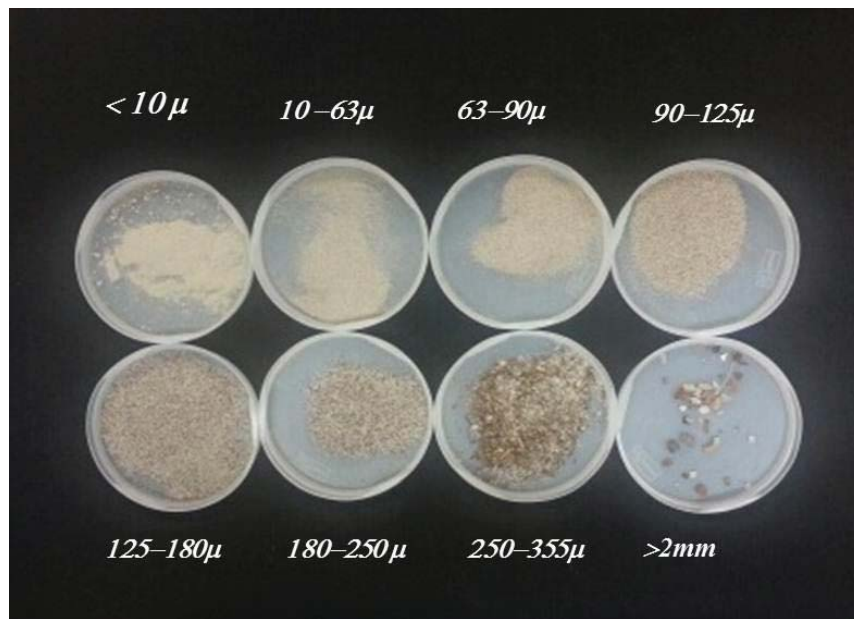
Figure 51. Image of near-field deposition after sieving into eight different size classes for chemical analyses.
