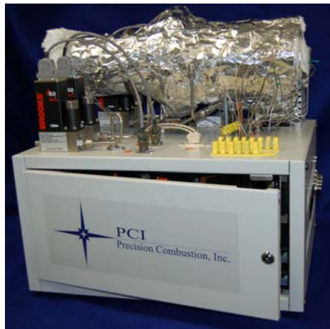
Figure 7. Photo of the integrated SDU prototype system with the downselected Sabatier reactor and all necessary BOP components.
