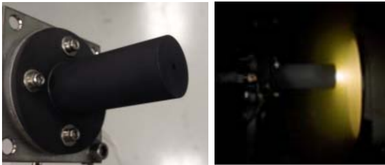
Figure 8. CSU delivered cathode and cathode operating on iodine.
