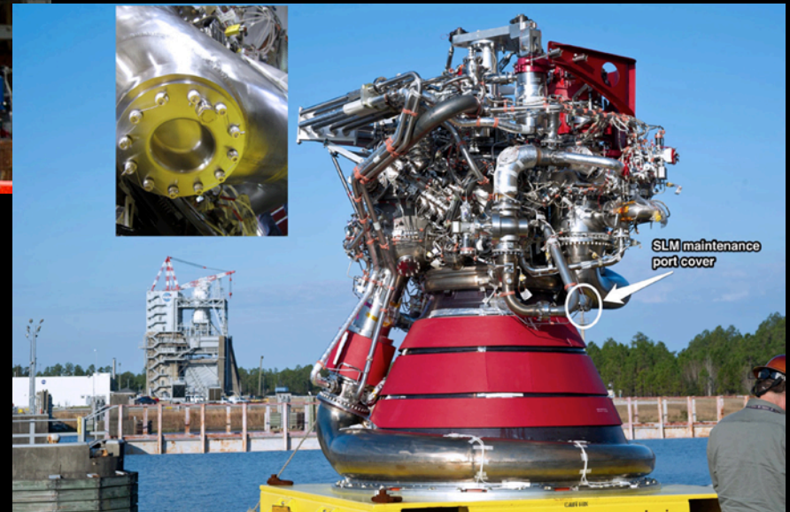
SLM Exhaust Port Cover for J-2X (inset and position on engine)
