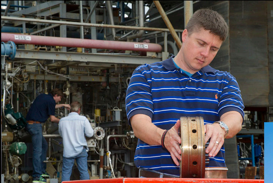
3-D printed rocket injector for hot fire test
