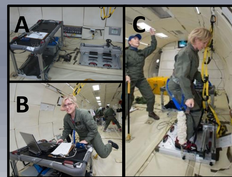
Figure 3: Parabolic Flight Test of XSENS ForceShoe™ A: Support console and test stand with static load force application device. B: Operator hovering over the support console and data acquisition system. C: Operator standing in the ForceShoes™ wearing the harness/bungee system.
