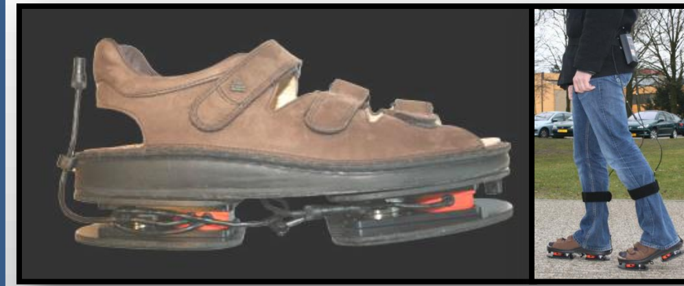
Figure 2: XSENS ForceShoe™ and instrumented subject.
