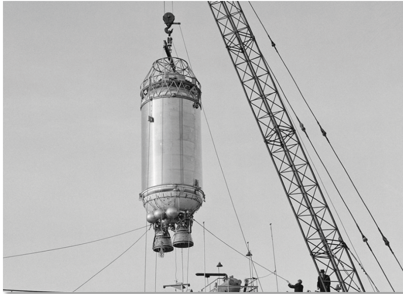
Figure 2. A Centaur stage being readied for testing.
