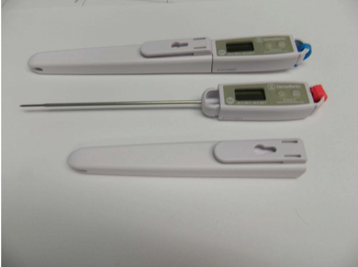
Figure 2.2-1. The two Thermoworks RT600C thermometers with color-coded identifying cable ties.
