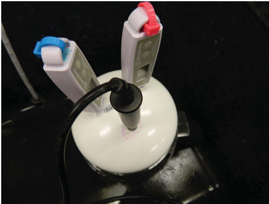
Figure 2.3.2-3. The assembled thermometer intercomparison bath.
