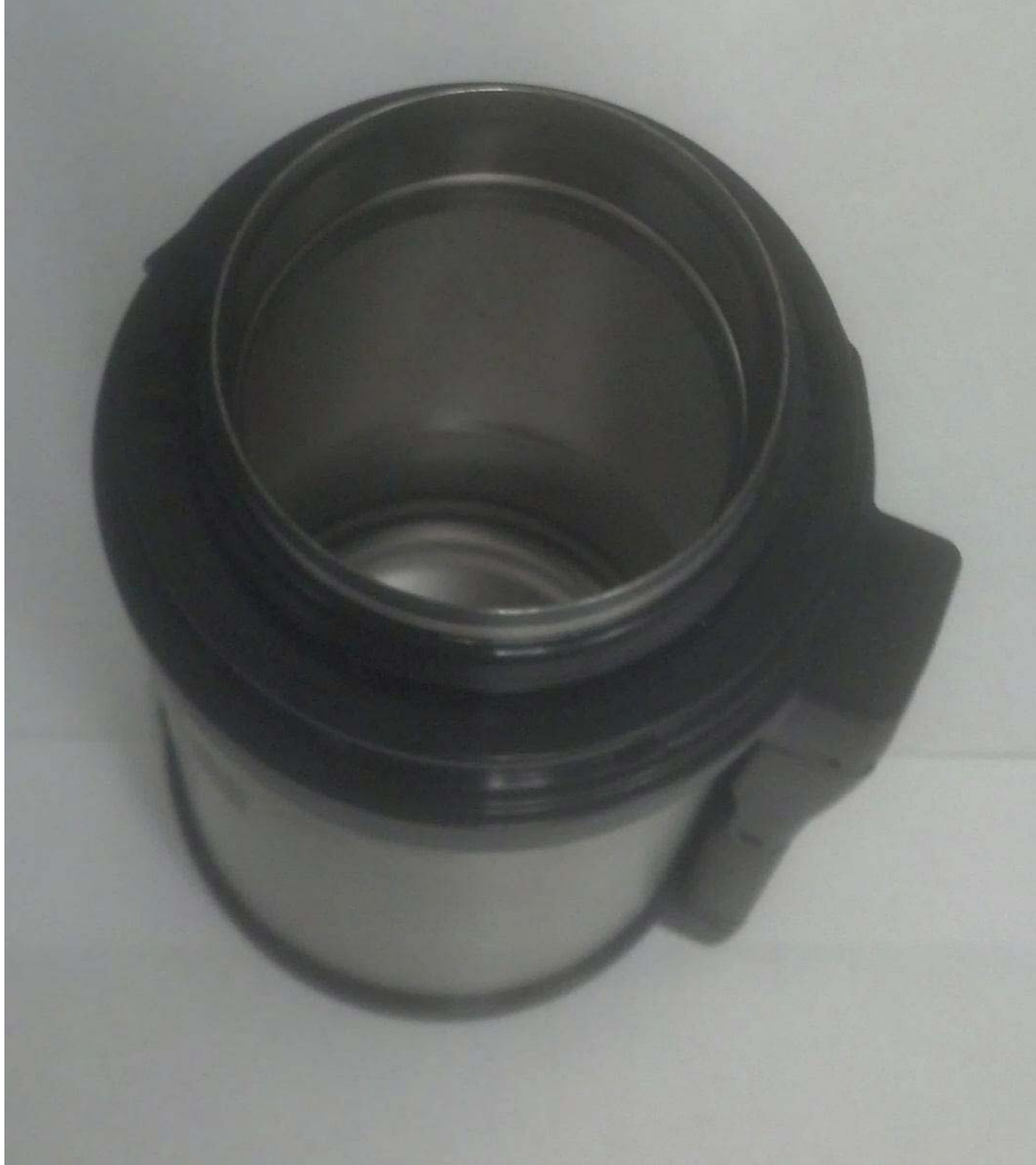
Figure 2.3.2-1. The body of the constant temperature bath.
