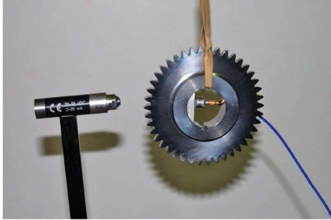
Figure 6.—Impact test setup (shown with steel gear).
