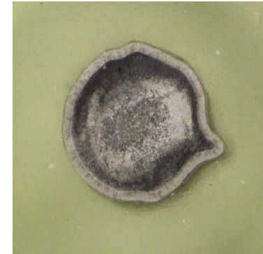
UO 2 agglomeration in current samples. Dark regions are UO 2 , light regions are W.
