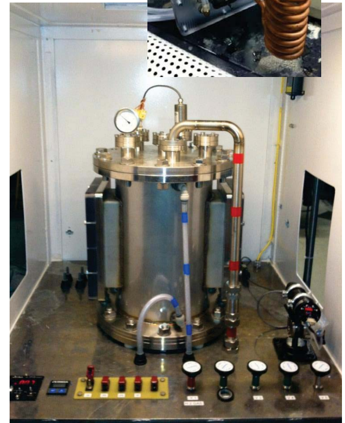
CFEET Chamber and RF Induction Coil
