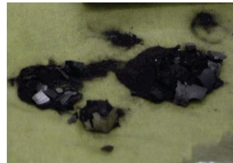
W-UO 2 slug after 10 min in CFEET at 2500C
