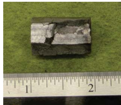
7-hole W-UO 2 in CFEET and post testing up to 2400 C
