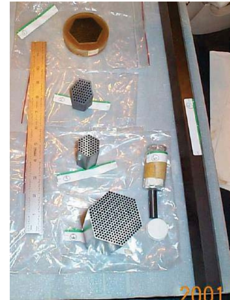
W-UO 2 CERMET Samples fabricated during ANL Program
