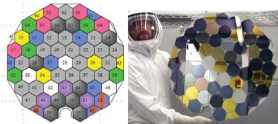
Fig. 1. (left) Pre-flight map of “B” array hexagonal collectors. Dark gray are CZ, light gray are FZ. (right) Person holding H array, for scale.
