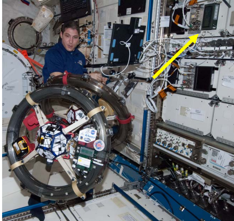
Figure 15. Multi-Gas Monitor operating in the JEM on ISS with SPHERES-RINGS nearby. NASA photo ISS038E045621
