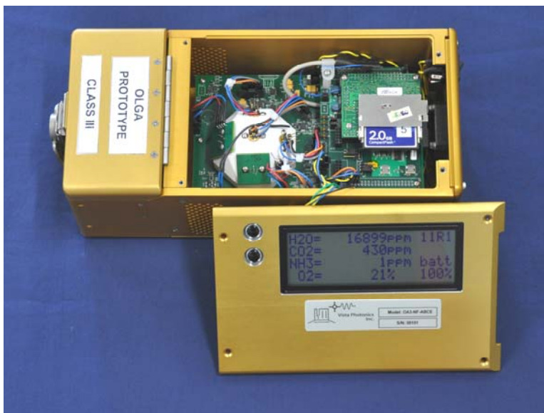
Figure 4. OLGA version 3.0. The custom FPGA board plugs directly into the main analog electronics board that controls the lasers. The sensor updates the significantly larger LCD and writes to file every 2.5 s, faster than the 7 s of earlier versions.
