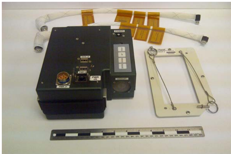
Figure 5. Sensor version 4.0, Multi-Gas Monitor. Flight prototype version 4.0 after assembly and integration. The adaptor plate allows for mounting to ISS equipment racks. The sensor can be powered through two USB ports or 28 VDC rack power.
