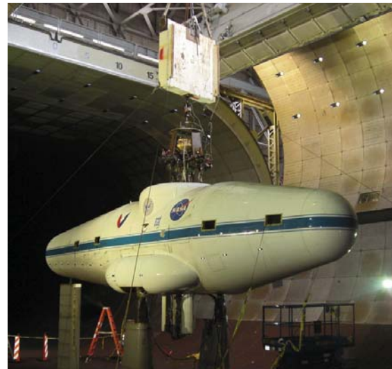
Figure 2. Shake test installation. Vertical shaking on the hub centerline
