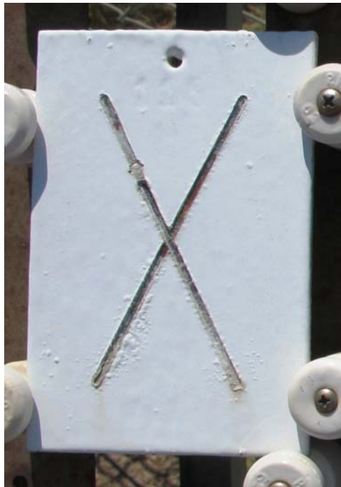
Figure 8: Undercutting from the Scribe for Sample from System 9
