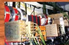
Heavy Ion Testing of Inflatable Shield Prototype
