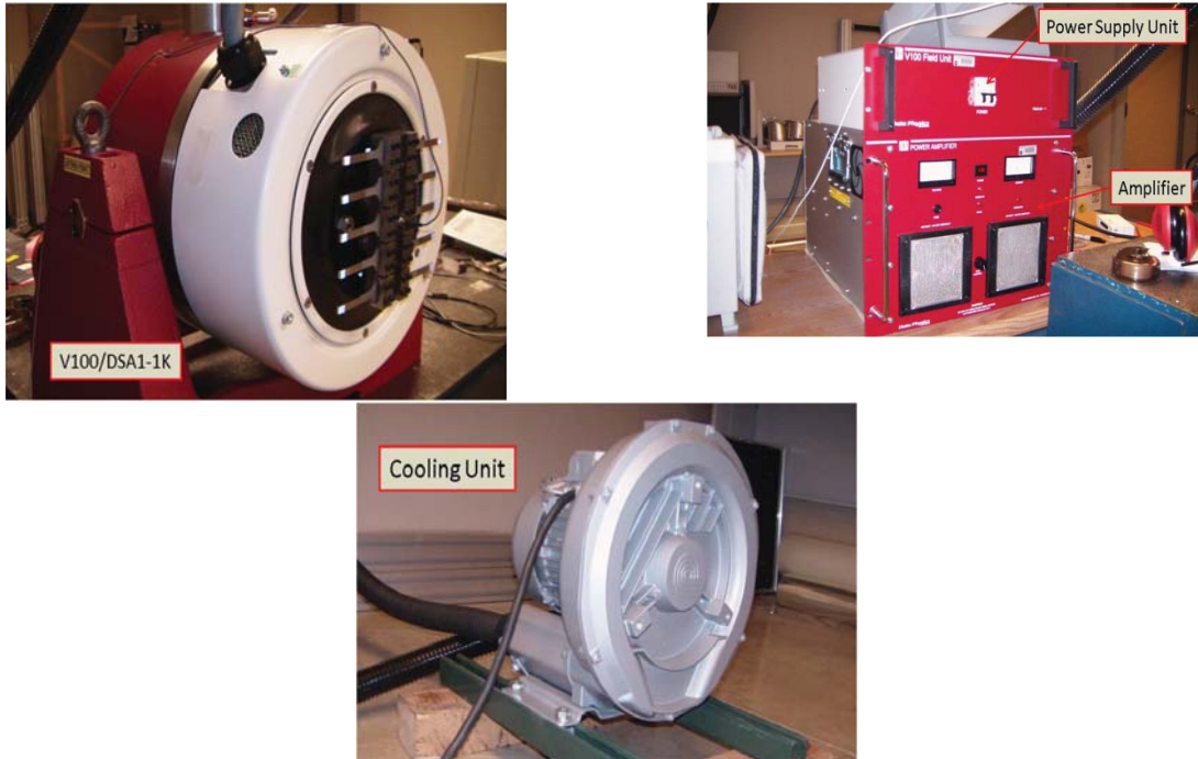
Figure 3.—DP shaker system.
