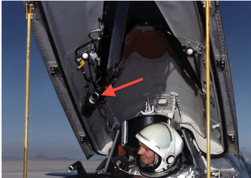
Figure B-7. Location of Film Camera on Canopy (DFRC)
