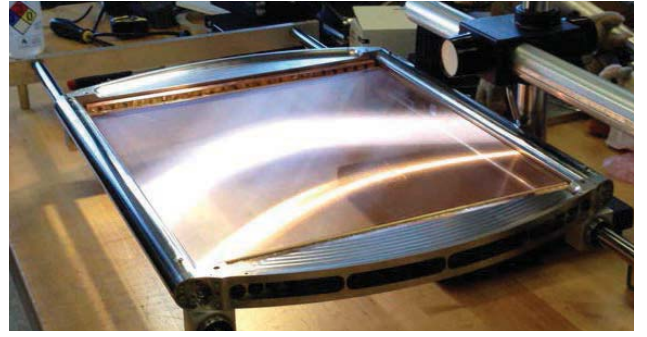
FIG. 5. The final cryogenically-compatible polarizing grid is shown. The dimensions of the grid are 41.7 \times 40 \text{ cm}^2 .
