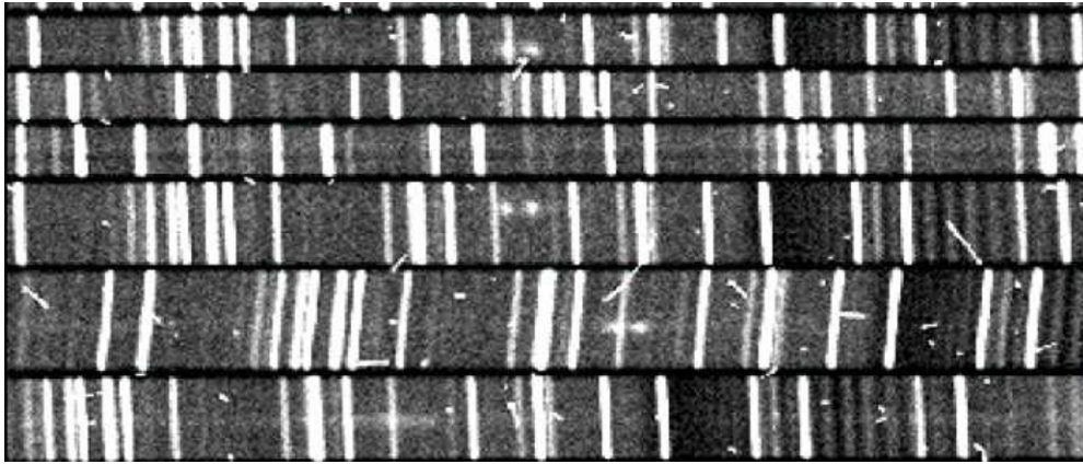
Figure 21. Section of single raw two-dimensional 20 minute exposure from the DEIMOS spectrograph. The [O II] doublet is visible in four objects, but cosmic rays and night-sky lines are much brighter than galaxy emission features.
