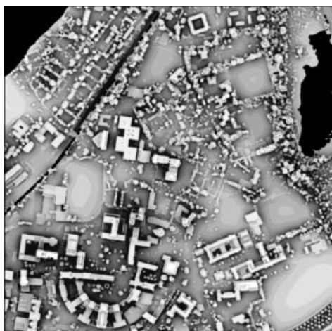
Figure 3. Spatial map of the sky view factor over the University of Birmingham study site. Note that the lidar data are not obtainable over water bodies, such as the lake in the upper right. The top left of the region is outside the coverage of the digital surface model (DSM) data.
