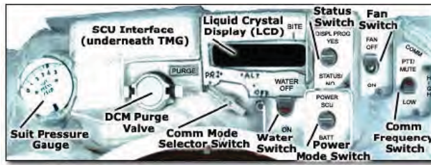
Figure 1. Power, Avionics and Control Software Critical Systems
