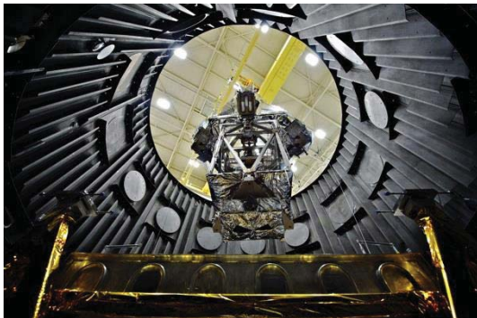
Figure 3. OSIM Bench being lowered into the SES
