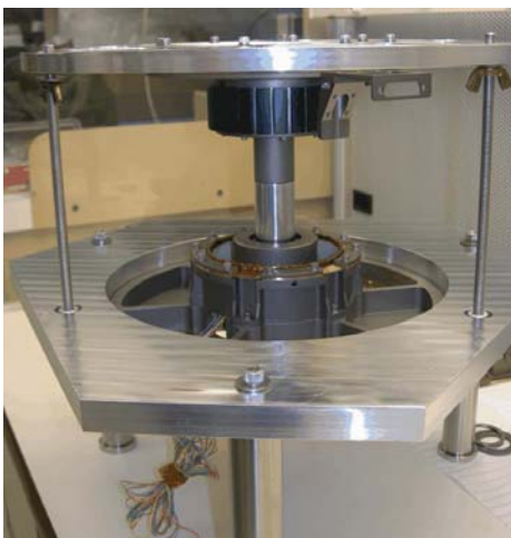
Figure 10: Motor Rotor Manually Lowered into Stator Assembly
