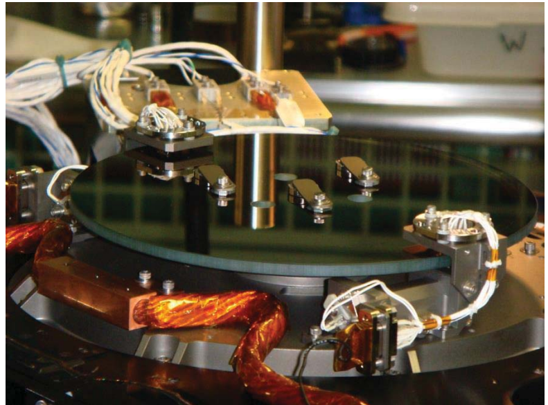
Figure 17. PSM Encoder Disk
