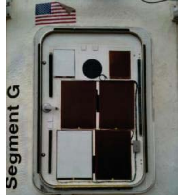
Dust Mitigation: Electrodynamic Dust Shield & Lotus Coating
