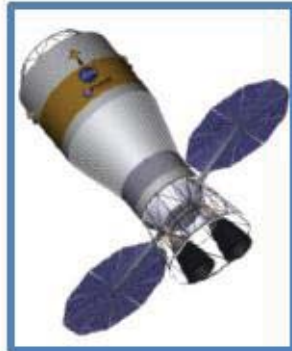
Cryogenic Propulsion Stage (CPS)
