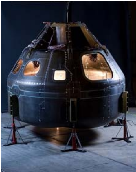
Figure 1. Image of NASA Composite Crew Module pressure vessel, showing an example of a complex geometry CFRP aerospace composite structure [4].
