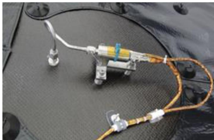
Figure 3. MEADS flight hardware installed on the MSL heatshield.
