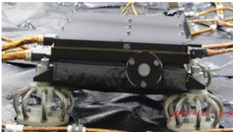
Figure 7. SSE box and WRI integrated on heatshield.
