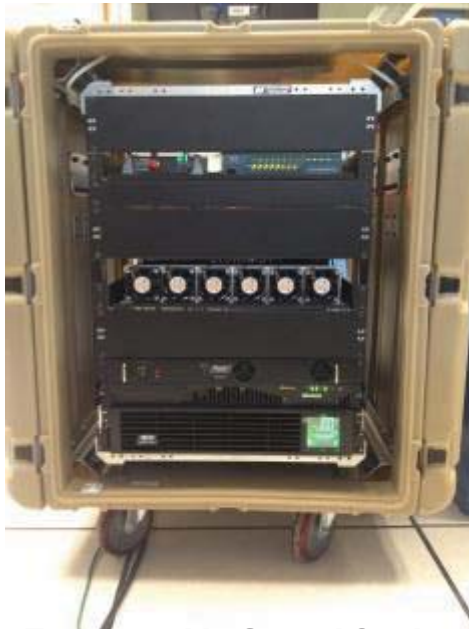
Transportable Ground Station
