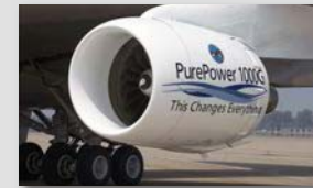
P&W PurePower 1000G Geared Turbofan
