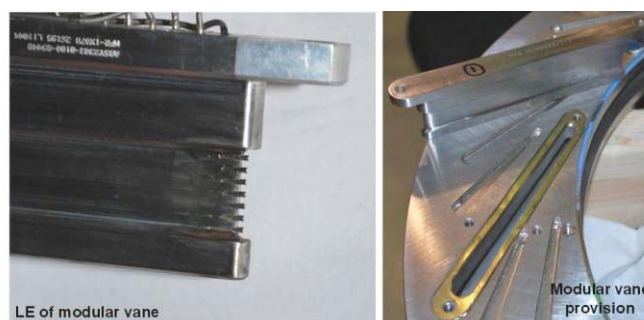
Figure 6. Leading edge Kiel head instrumentation on main diffuser vane
