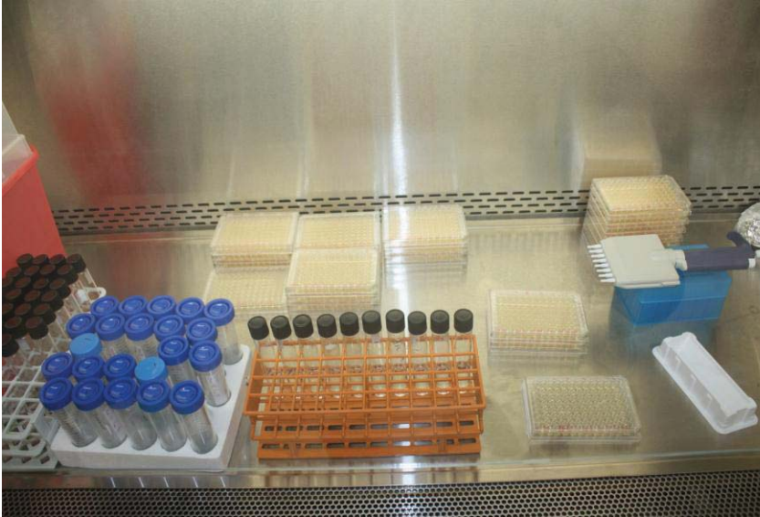
Figure 5. MPN setup. Blue Falcon tubes contained the treated spore coupons. The rack was stocked with test tubes that were filled with 9 mL of sterile DI water for the serial dilutions. The 96-well plates were labeled and filled with MPN spore media. The spores were diluted in and each dilution was placed in 16 wells of the plate with a multi-channel pipette with well boats such as the one on the right of the image.
