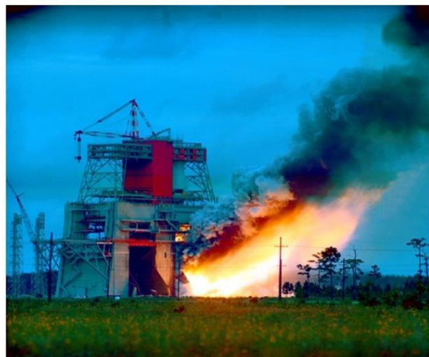
Static Firing Test Stand at MSFC (No Side Deflector or Water System)
