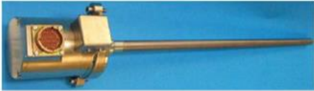
Figure 3: Sample Cartridge Assembly (SCA), in which a sample for a directional solidification experiment on the ISS is contained.
