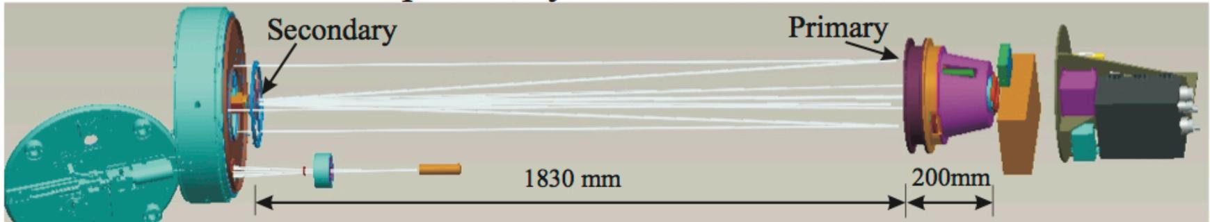
Primary to secondary requirements: Distance:  $\pm 0.05\text{mm}$
