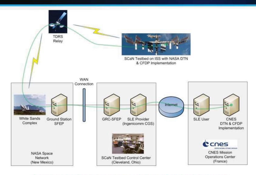
End-to-end data flow between CNES and NASA's ground and space assets using space internetworking protocols
