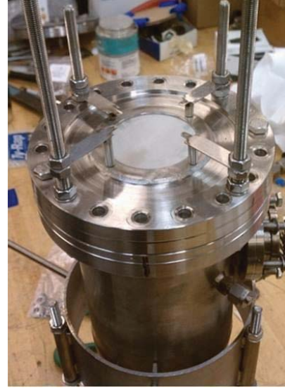
Fig. 7 Completed LAD Screen/Cup Assembly
