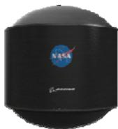
*NASA has completed a complex series of tests on one of the largest composite cryogenic fuel tanks ever manufactured, bringing the aerospace industry much closer to designing, building, and flying lightweight, composite tanks on rockets.*
