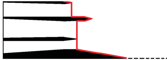
Figure 9. 2D-axisymmetric gross thrust control surface (shown in red), Configuration 1.
