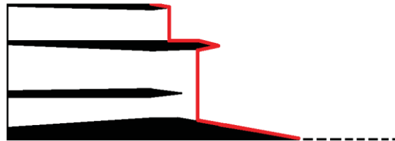
Figure 10. 2D-axisymmetric gross thrust control surface (shown in red), Configuration 1.5.
