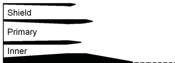
Figure 1. Generic three-stream nozzle geometry (axisymmetric cut).
