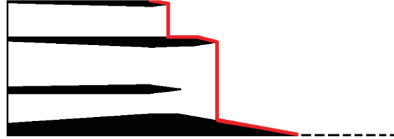
Figure 11. 2D-axisymmetric gross thrust control surface (shown in red), Configuration 2.
