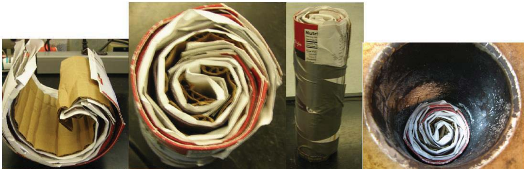
Figure 3. Assembled densely packed cardboard footballs.
