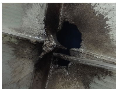
Close-up of simulated MMOD Damage to External ISS Panel
