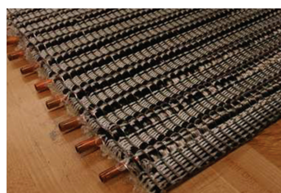
Carbon fiber radiator design
