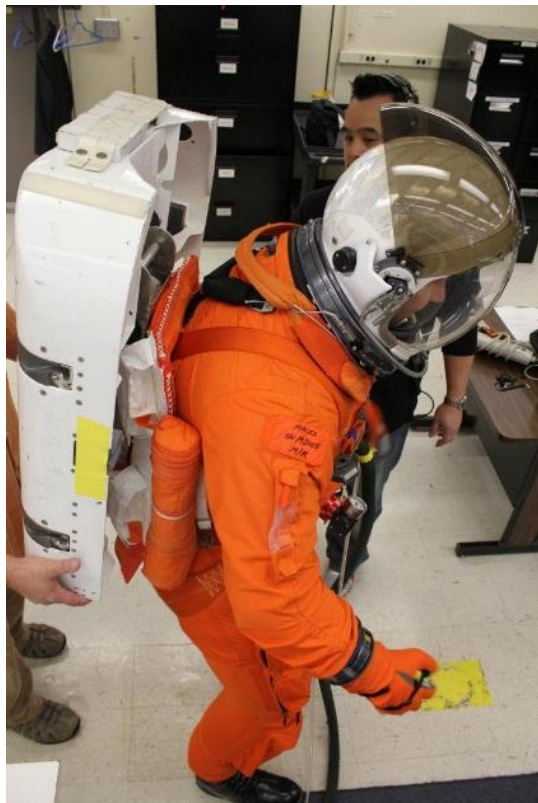
Figure 2 EMU PLSS Simulator Mounted on MACES
