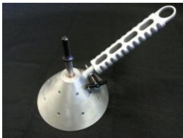
Figure 9 Bell & Chisel Sample Collection Device
