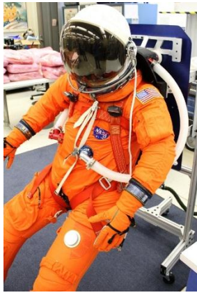
Figure 16 Pressurized MACES and Interface Kit
