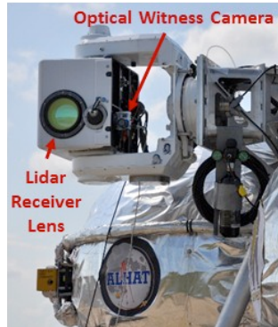
Figure 7. An optical witness camera with larger FOV than the HDS FL provides additional situational awareness in post-flight data analysis and in pre-flight checkouts.
