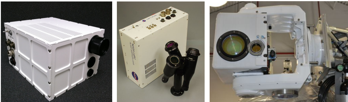
Figure 1. Prototype ALHAT sensors flight tested on Morpheus in 2014: long-range LAlt (left), NDH optics head and electronics (center), and HDS gimbaled flash Lidar (right).
