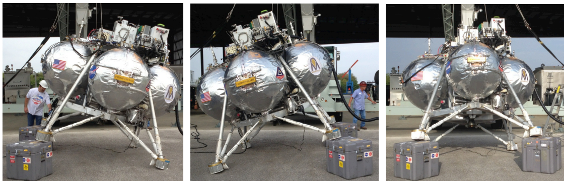
Figure 6. Tilt tests of integrated Morpheus vehicle with ALHAT Hazard Detection System to compare gyro orientations with metrology measurements.
