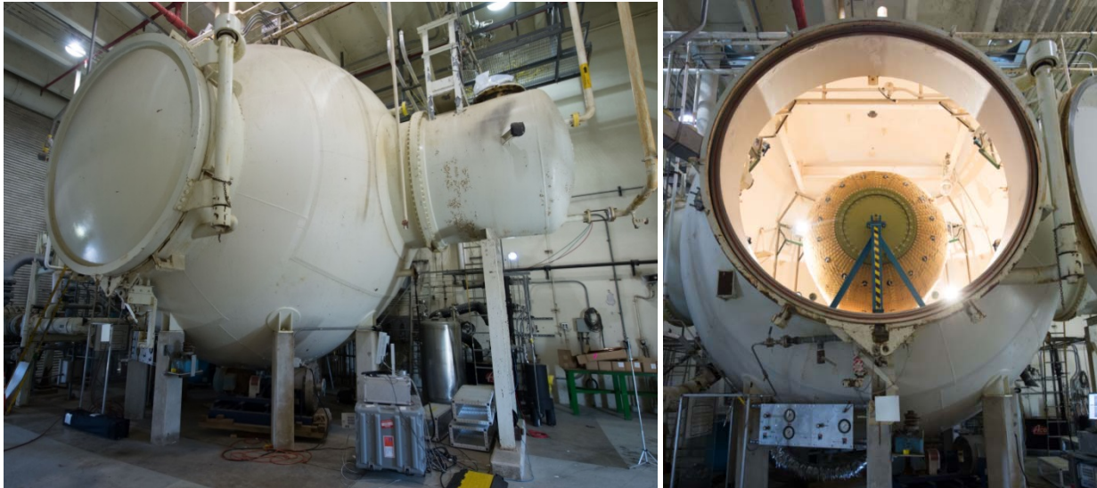
Figure 6. The test chamber at the JSC Energy Systems Test Area where the Creep Burst Test was performed.
