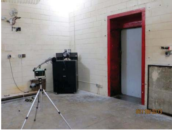
Figure 7: RAL's ASTM-E90 TL Test Setup
