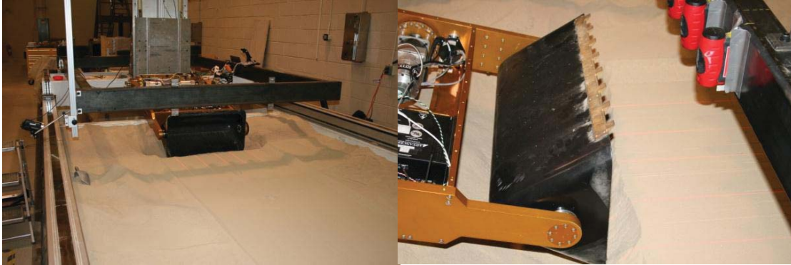
Figure 5. Excavator lowered to desired depth and rake angle pre-test.
