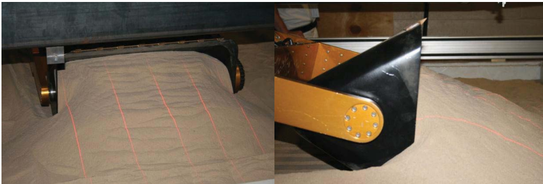
Figure 6. Soil pile-up with laser profiling post-test.
