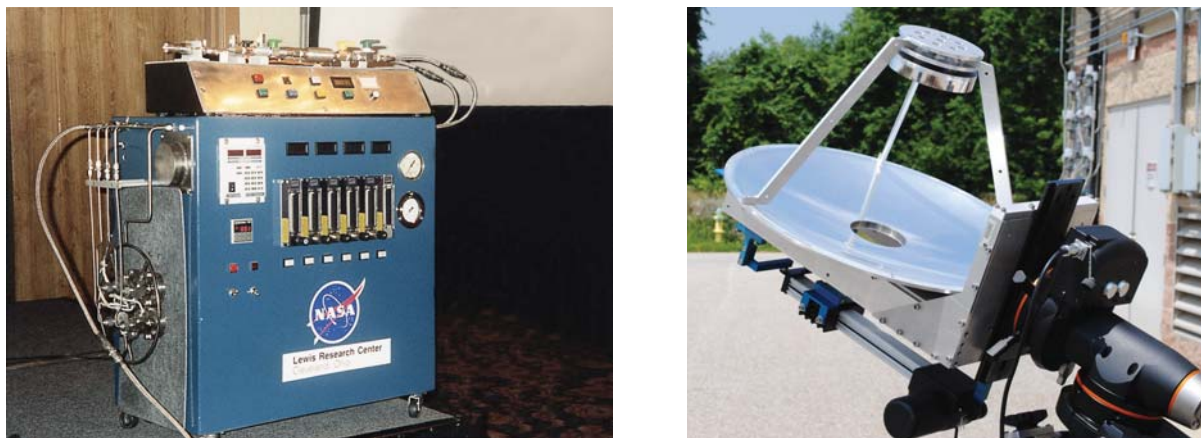
Figure 4.—Two example ISRU technologies at GRC—(left) Mars CO propellant production plant and (right) solar concentrator for processing regolith simulant.
