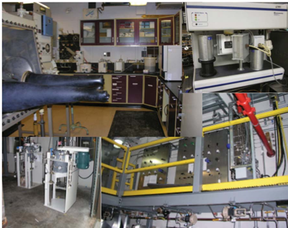
Figure 3.—Example facilities for processing catalysts, characterizing, and screening fuel production catalysts; from upper left-hand corner: synthesis laboratory, instrument for TPR analysis, Alternative Fuel processing Facility, and continuously-stirred tank reactor.
