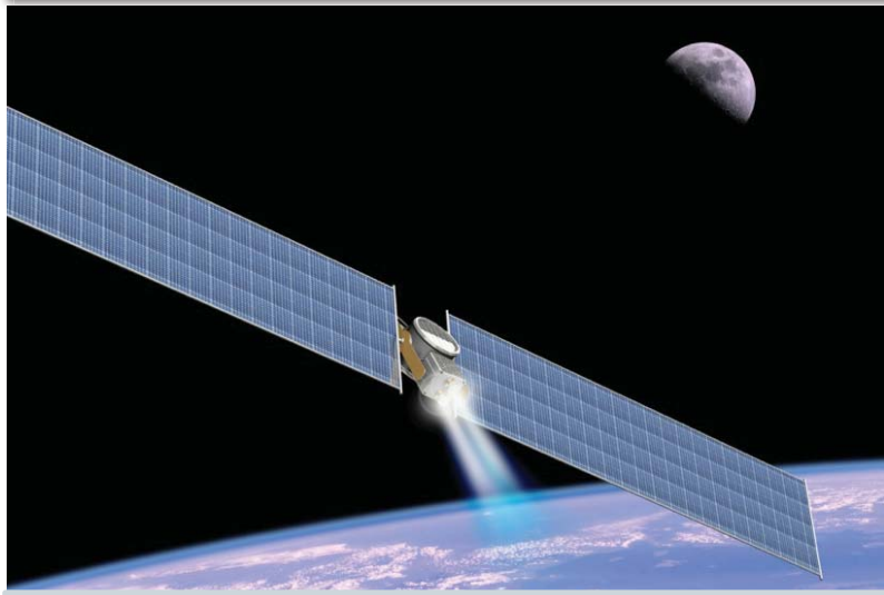
SEP vehicle initial launch mass of 1/2 Falcon 9 performance to GTO (2800 kg)
