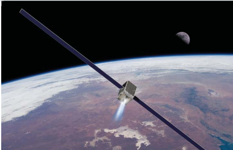
SEP vehicle initial launch mass of 1/2 Falcon 9 performance to GTO (2800 kg)
