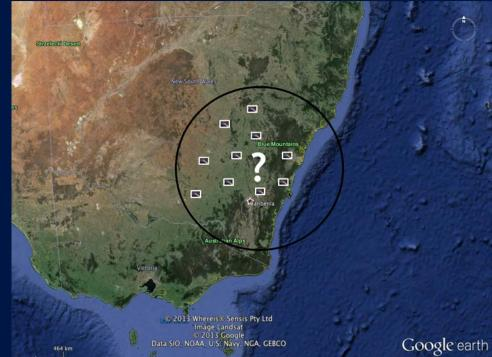
Astronaut photography from ISS is collected using COTS digital cameras with no native geolocation information. Camera look direction and viewing angle is unconstrained (left image); therefore the ISS nadir point is only useful as a starting geographic reference point.
